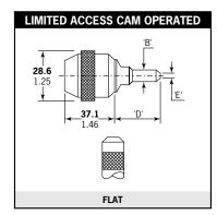
Available as shown in NOSE JAW SELECTION TABLE overleaf. Equivalent functions to the Standard and Limited Access above with the addition of a cam to ease and speed up the nose jaw opening thus the pod reloading procedure.
